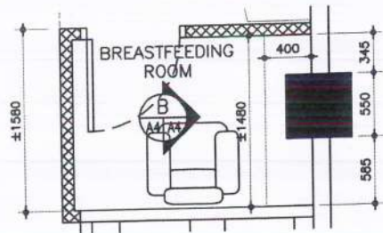
A BREASTFEEDING ROOM BLOW-UP PLAN SCALE 1:50 MTS
