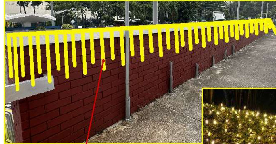
WARM WHITE OUTDOOR LED CURTAIN WALL LIGHTS (500-700M LENGTH, SPACED AT 100-150MM)
